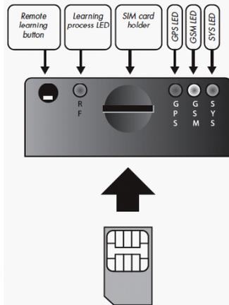
5. Wait until both the yellow GSM LED and the green SYS LED are flashing. The red GPS LED should be on, steady or flashing, depending on whether it has established contact with the GPS satellites. In other words, all LEDs are flashing when the system is activated! (You don't have to wait for the red LED to start flashing before you go to step 6.) **Note!** The red GPS LED should have started to flash within 60 minutes from activating the alarm.
